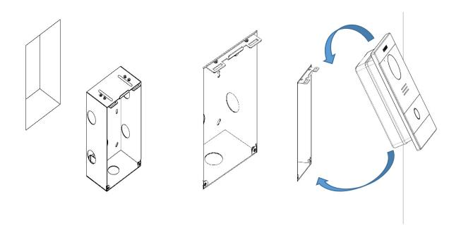
○,1Flush box insta ○,2Base flush box depth adjustment hook ○,3The upper part of the panel is stuck in, then move the panel to the flush box.
