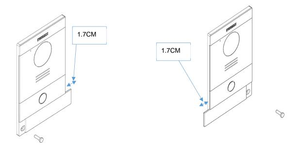
O,4Move the slider of the panel and fix the two screws, when installing, pay attention to the reservation of the 1.7CM space around the door to move the slide cover.
