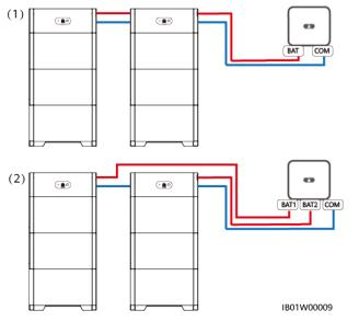
Figure 6-18 Battery cascading cable connection (two batteries)
