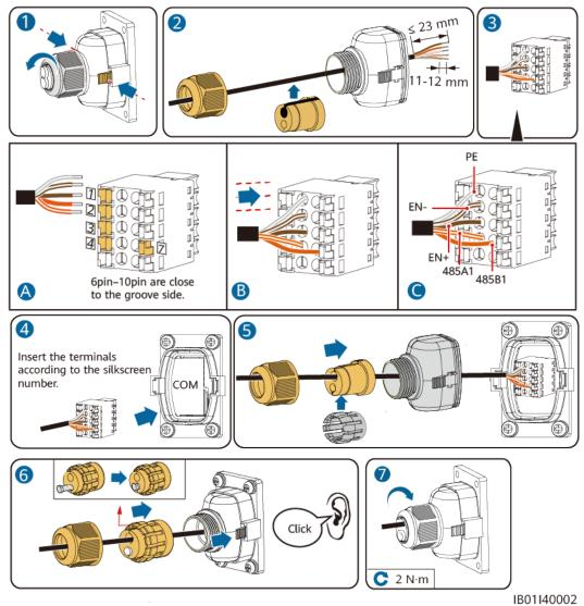
Figure 6-17 Connecting inverter terminals
