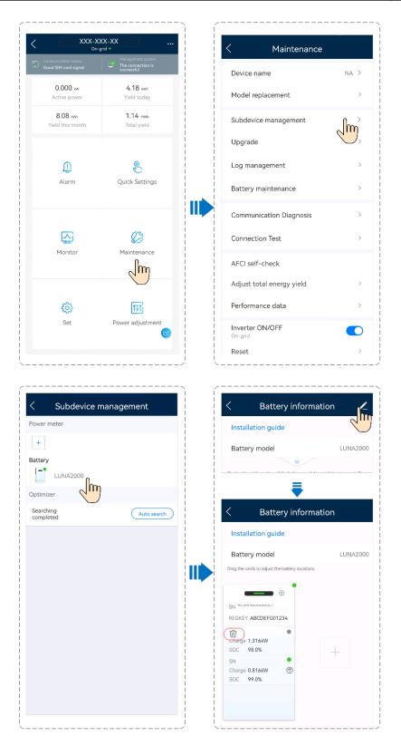
When the EMMA is used for networking, **connect to the EMMA on the app**, tap **Monitor** on the home screen, select the connected inverter, choose **Maintenance** > **Subdevice management**, tap the ESS icon, and delete the offline power control module or battery expansion module.
