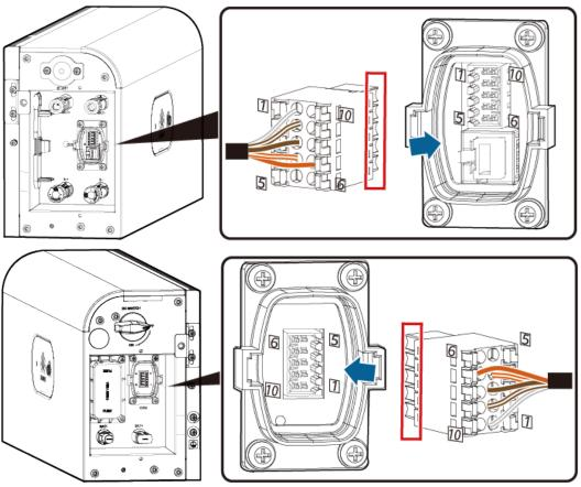
Figure 6-16 Inserting the terminal
