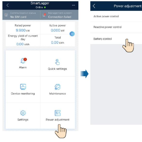
Figure 7-12 Setting the battery working mode
