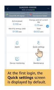
Step 2 Tap Quick settings to set parameters for commissioning as prompted. For details about setting the battery working mode, see 3 "Application Scenarios and Settings".
