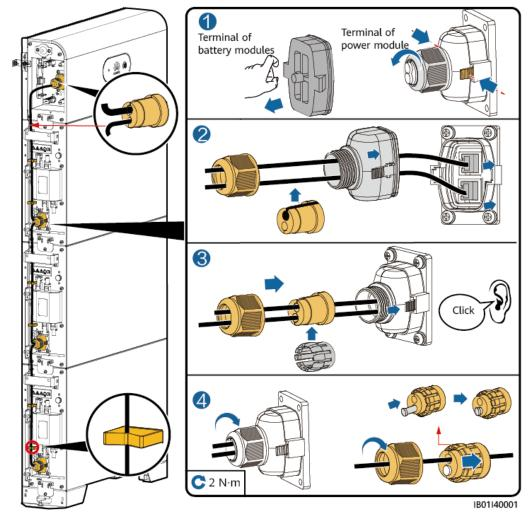
Figure 6-6 Securing With Clips
