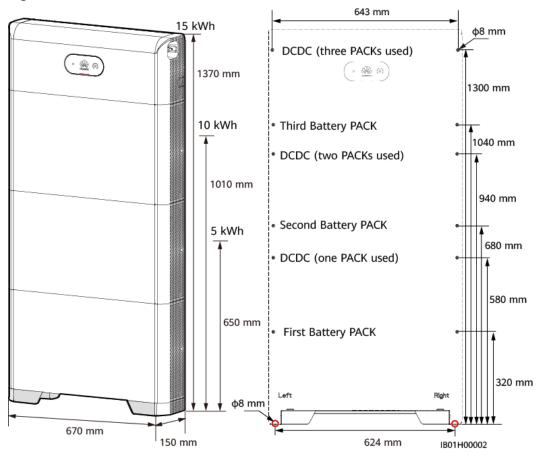
Figure 5-2 Floor-mounted installation dimensions
