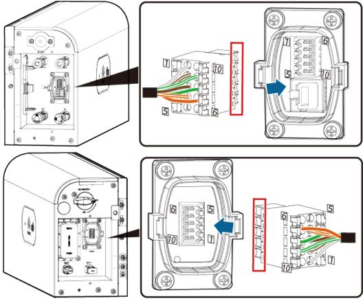
Figure 6-21 Inserting the terminal
