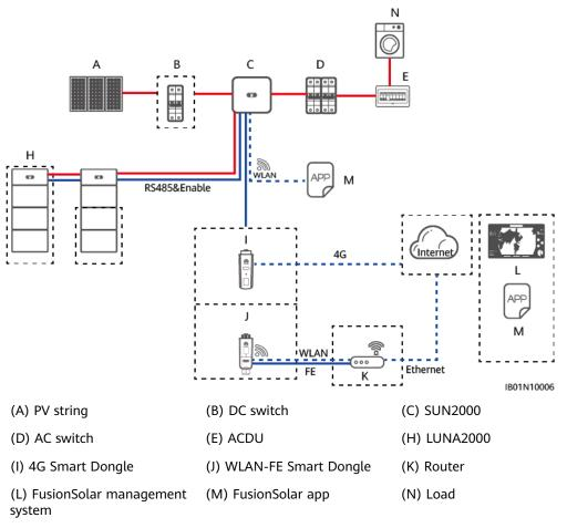
Figure 4-15 Off-grid ESS (dashed boxes indicate optional components)
