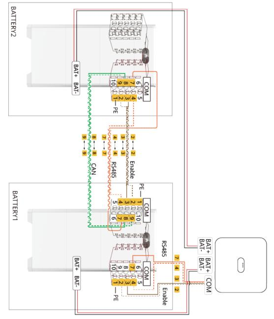
Figure C-3 Inverter connected to two batteries (method 2)
