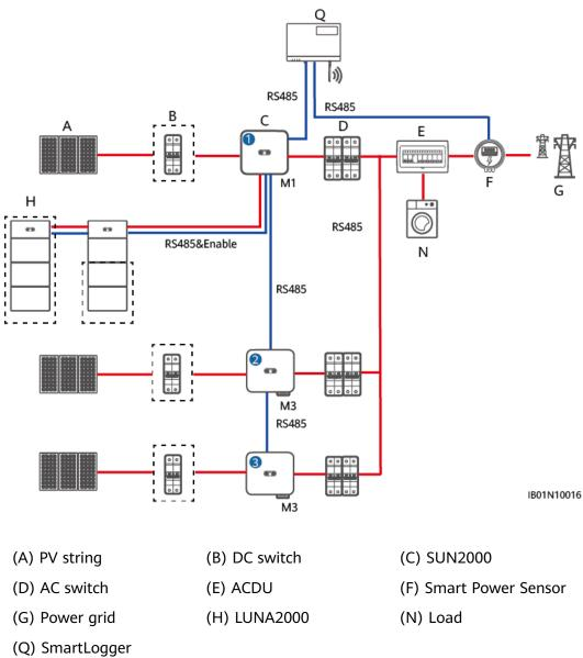
**Figure 4-2** Networking of one SUN2000-(3KTL-10KTL)-M1 and two SUN2000-(20KTL, 29.9KTL, 30KTL, 36KTL, 40KTL)-M3 inverters (dashed boxes indicate optional components)
