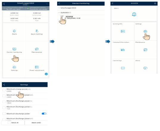
Figure 7-13 Setting the battery parameters
