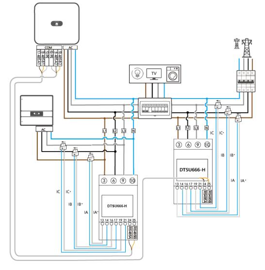
Figure 4-19 Power meter cable connections for SUN2000-(3KTL-10KTL)-M1
