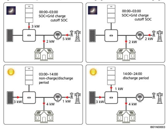
Figure 4-9 Example of TOU (00:00–03:00 charging and 14:00–24:00 discharging)
