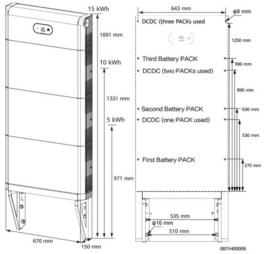
Figure 5-7 Wall-mounted installation dimensions
