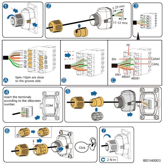
Figure 6-22 Cascading communication terminal
