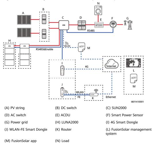
Figure 2-5 Networking (dashed boxes indicate optional components)
