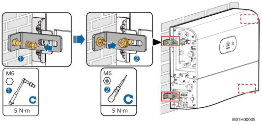
Figure 5-6 Fixing the power control module
