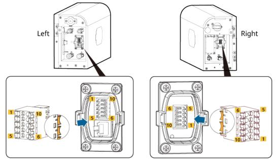
Figure C-1 Insertion direction of a battery communications terminal
