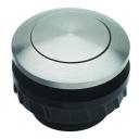
Klingeltaster, Edelstahl V2A/Stainl. St., max. 12V AC /= (AC/DC)/1,5A, Ø16mm, Platte/plate 1-6mm, IP 54,
