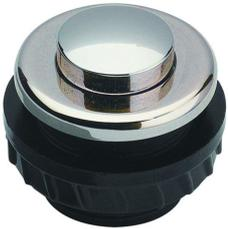
Klingeltaster, MS vernick./Brass Ni pl., max. 12V AC /= (AC/DC)/1,5A, Ø16mm, Platte/plate 1-6mm, IP 54,
