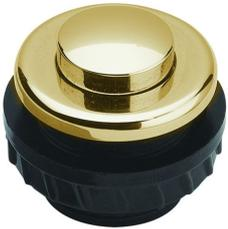
Klingeltaster, MS vergold./Brass gold p., max. 12V AC /= (AC/DC)/1,5A, Ø16mm, Platte/plate 1-6mm, IP 54,
