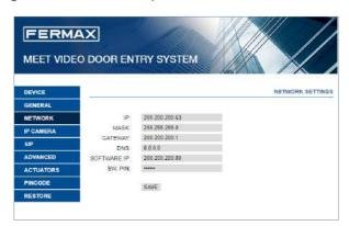
**IP:** IP address to be assigned to this monitor. **MASK:** Subnet mask corresponding to the LAN
