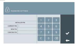
Use the numeric keypad to identify yourself with the current PIN and enter the new PIN. Confirmation of the new PIN is requested for security purposes.
