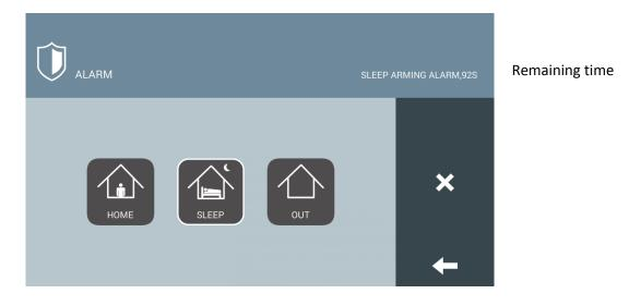
The change will be made automatically after 100 seconds to prevent the alarm from being triggered if you need to pass through the protected area. The remaining exit time is displayed.
