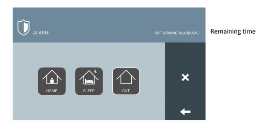
Once the time has elapsed, the monitor will return to the standby screen, displaying an icon indicating the current mode in the upper left corner.
