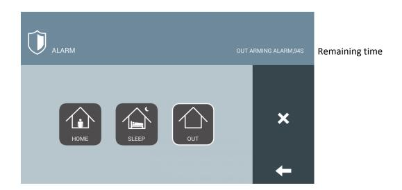
Once the time has elapsed, the monitor will return to the standby screen, displaying an icon indicating the current mode in the upper left corner.
