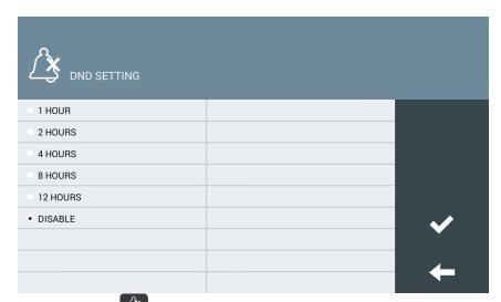
Touch the icon to activate the Do Not Disturb option and set the required time between 1, 2, 4, 8 or 12 hours, or to deactivate it before the programmed time has elapsed.
