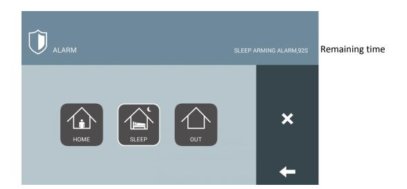
The change will be made automatically after 100 seconds to prevent the alarm from being triggered if you need to pass through the protected area.
