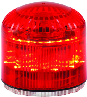
SIRENA SIR-E LED MAX blink/dauer + akustik, rot, IP65, 115 dB
